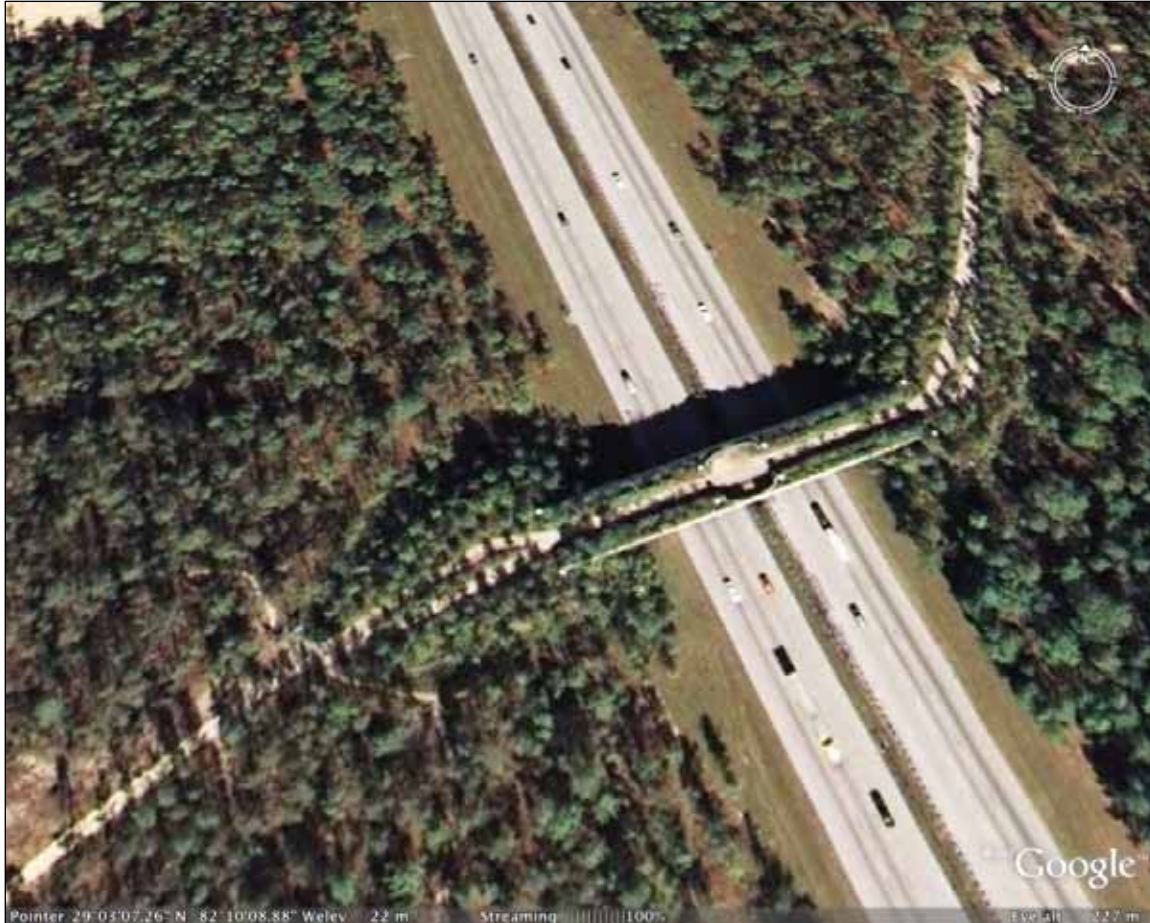
Figure 2. Photo. Wildlife crossings are becoming more common in highway expansion projects in North America. An example is the Greenway Landbridge on Interstate 75 in Marion County, Florida (Credit: Google Earth).
